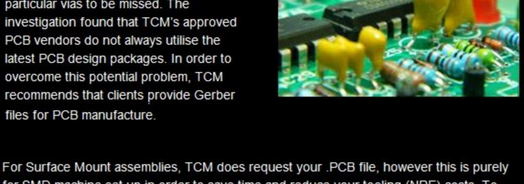
.PCB File – TCM SMD Machine programming only. Gerber File – PCB Manufacturing file.
